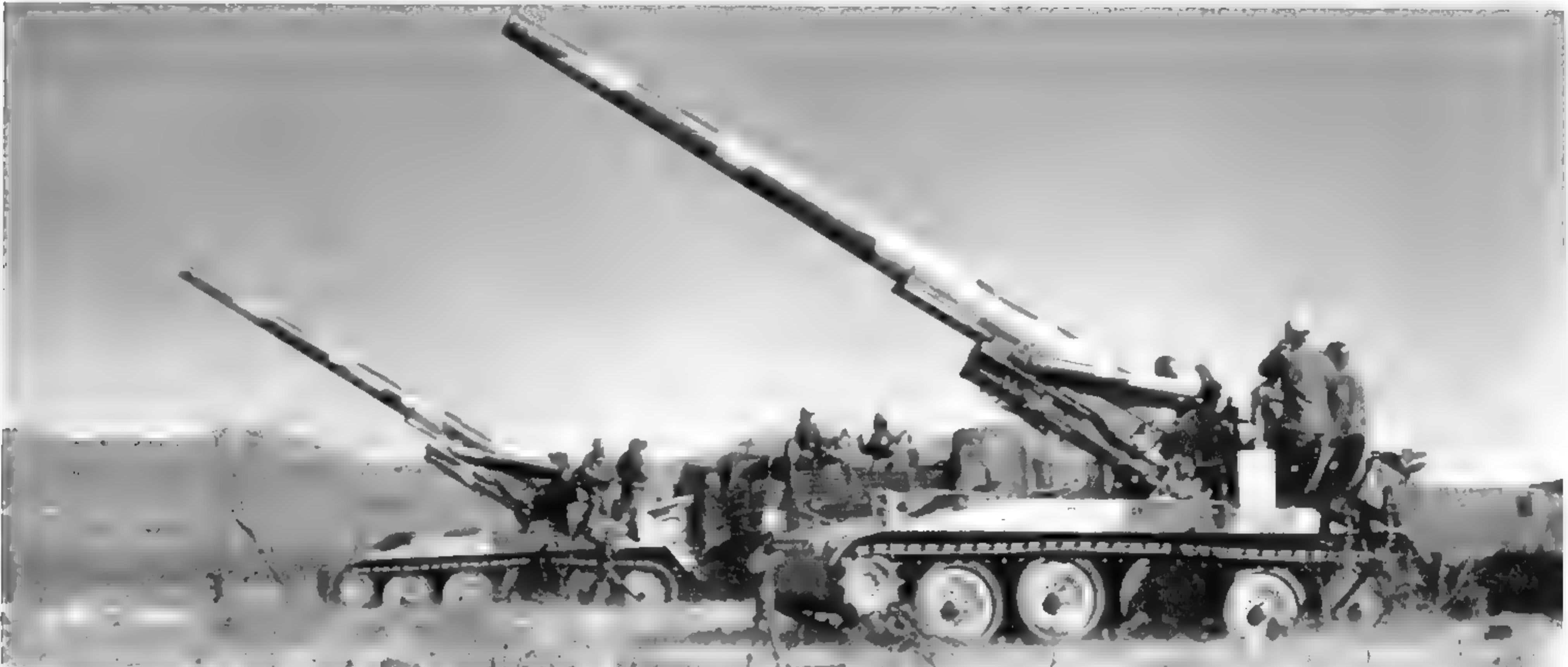
The M110A1 featured a longer howitzer than the M110, but still nowhere near the length of the M107's gun. These camouflage painted M110A1s are conducting a firing exercise in this view. (U.S. Army photo)
